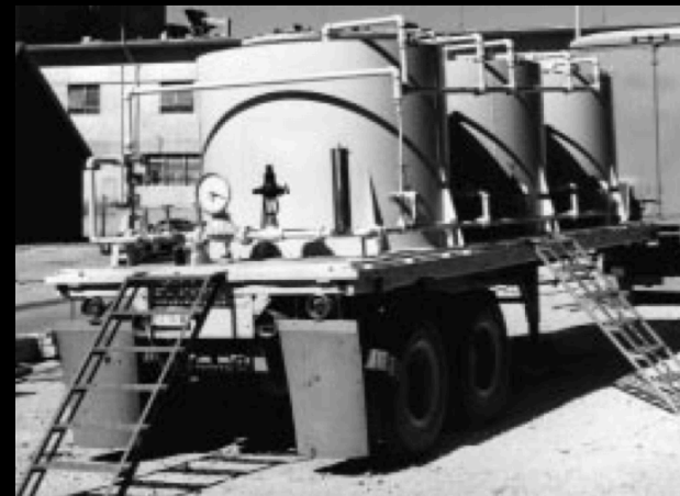
fluid handling system (4,500 l steel tanks)
