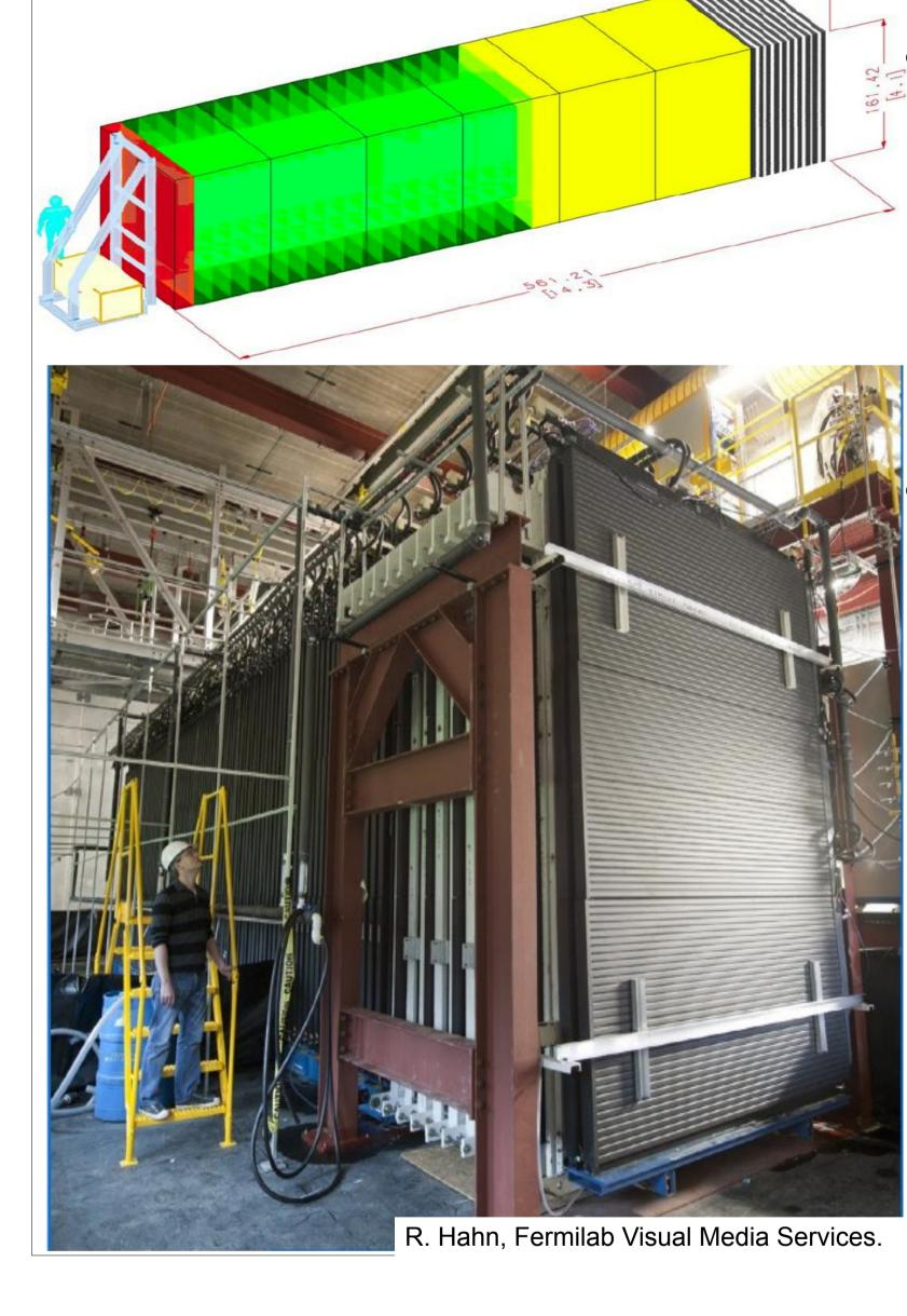
• The NDOS is located on the surface between the MINOS and MiniBoone experiments. It is 14m long, 3m wide, and 4m tall.
