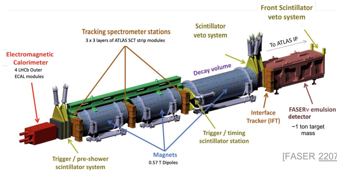
1 ton **FASERv tungsten emulsion detector** for neutrino measurements. Also target for electronic measurements using muon appearance.
