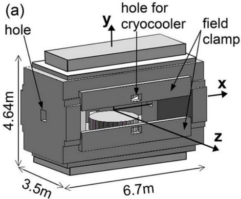
Key component of FASER2 is a large area, air core superconducting dipole magnet.
