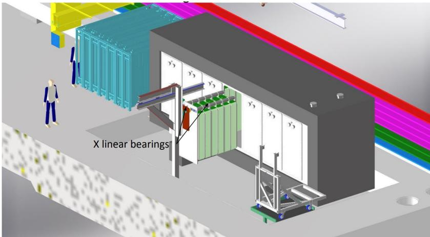
Installation sequence of TPCs into cryostat studied.
