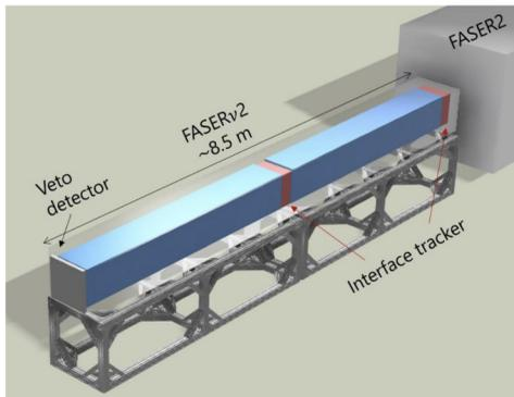
**FASER2:** tracking spectrometer for LLP searches and muon charge ID
