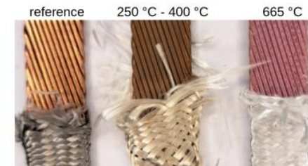
Fig. 4. Images of Rutherford cables after the RHT, with and without the introduction of oxygen.
