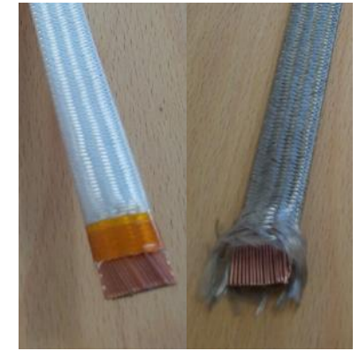
Nb 3 Sn Precursor Cable Insulated with S-2 Glass Before (Left) and After (Right) Nb 3 Sn Reaction Cycle (Courtesy of C. Urscheler)
