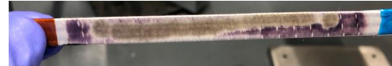
Iodine Test after Plasma Desizing of S2 Glass (636). 1mm Distance, 1.5m/s Moving Nozzle
