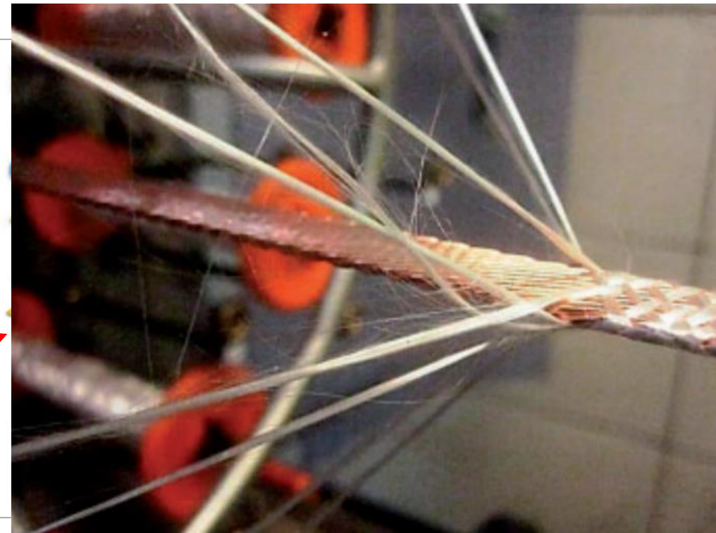
Image from Roy, S. S. et al. Braiding Ultrathin Layer for Insulation of Superconducting Rutherford Cables (2018) ( sagepub.com )
