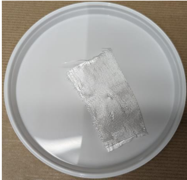
Appearance following Thermal Desizing
