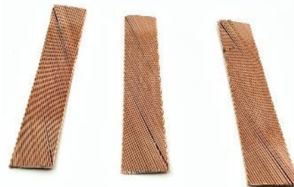
Cable conductor after plasma treatments above
