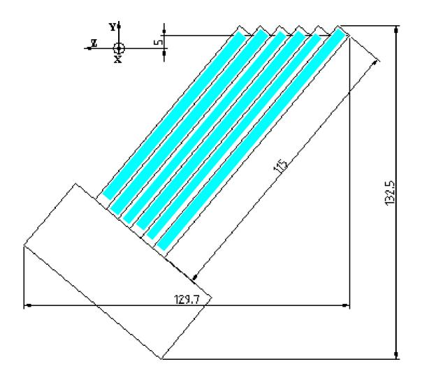
•Sawtooth easier to fabricate •6 rods in z •New drawing to evaluate dimensions (min z in baseline design is 130 mm).
