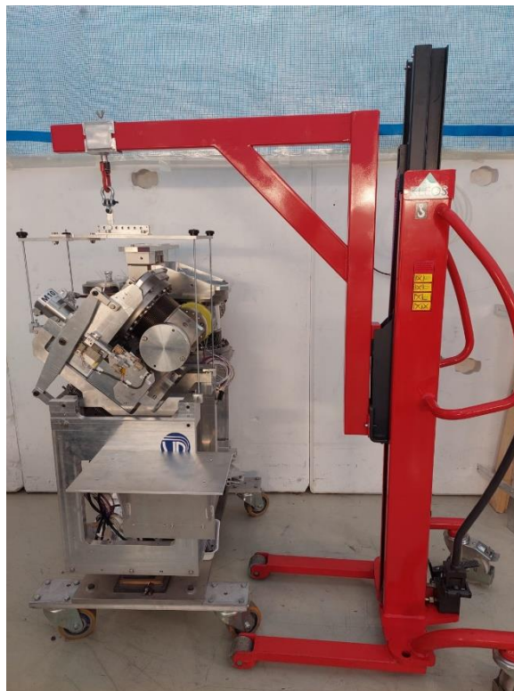
Figure 5: Top: sequence of operation for horizontal XRP rotation. Bottom: Mounting tool used in the LHC tunnel to lift the horizontal XRP.
