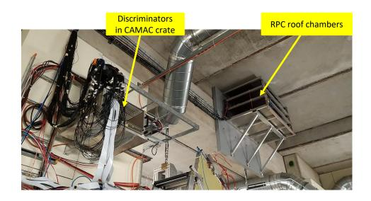
Signals from RPC chambers discriminated in a crate inside the bunker
