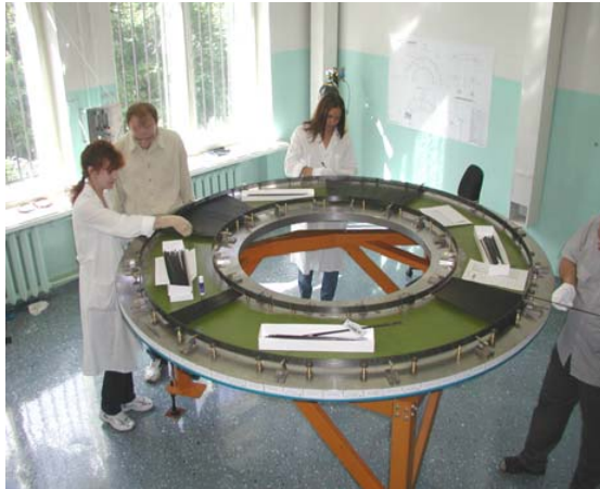
Installation of straws (tests leak tightness)
