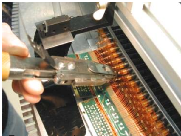
Fixating and connecting wires (tests wire tension & HV)
