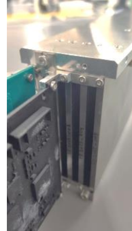
FoCal-E segment mockup w/ Tungsten
