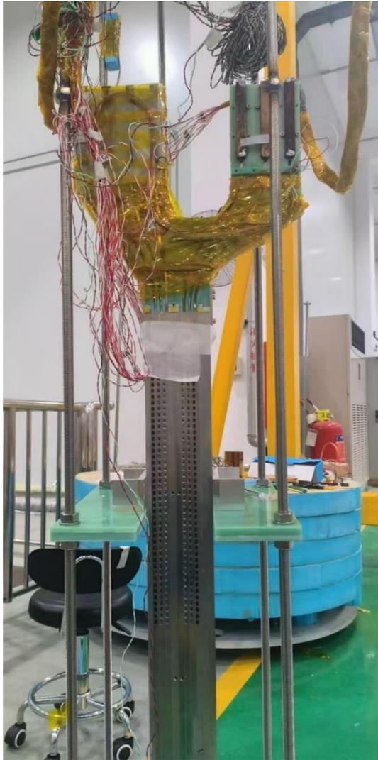
HTS insert coil after assembly
