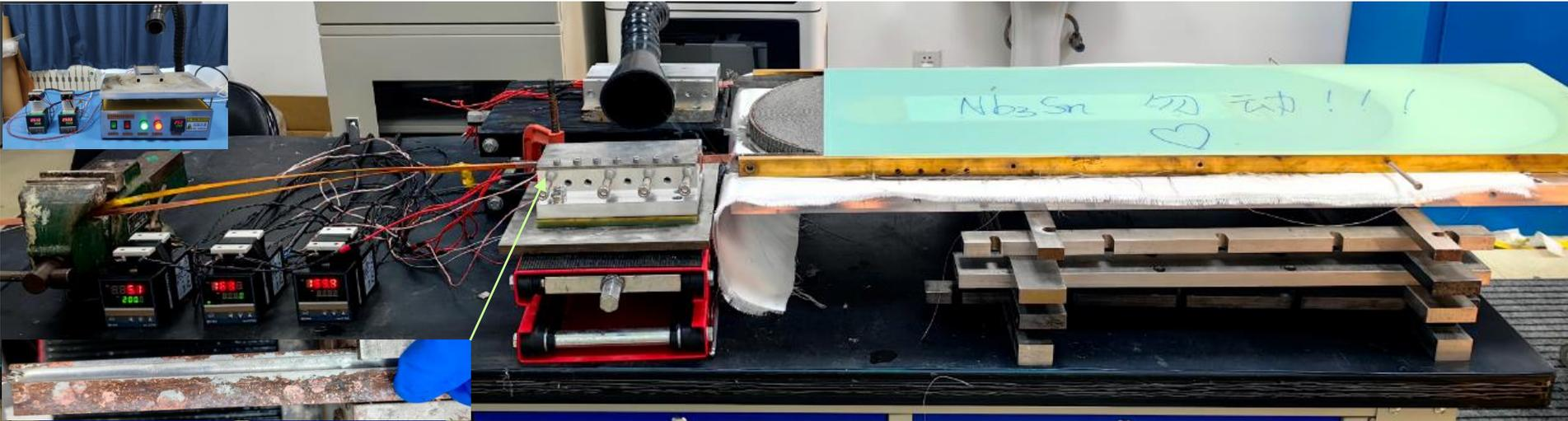
NbTi & Nb<sub>3</sub>Sn joints soldering system
