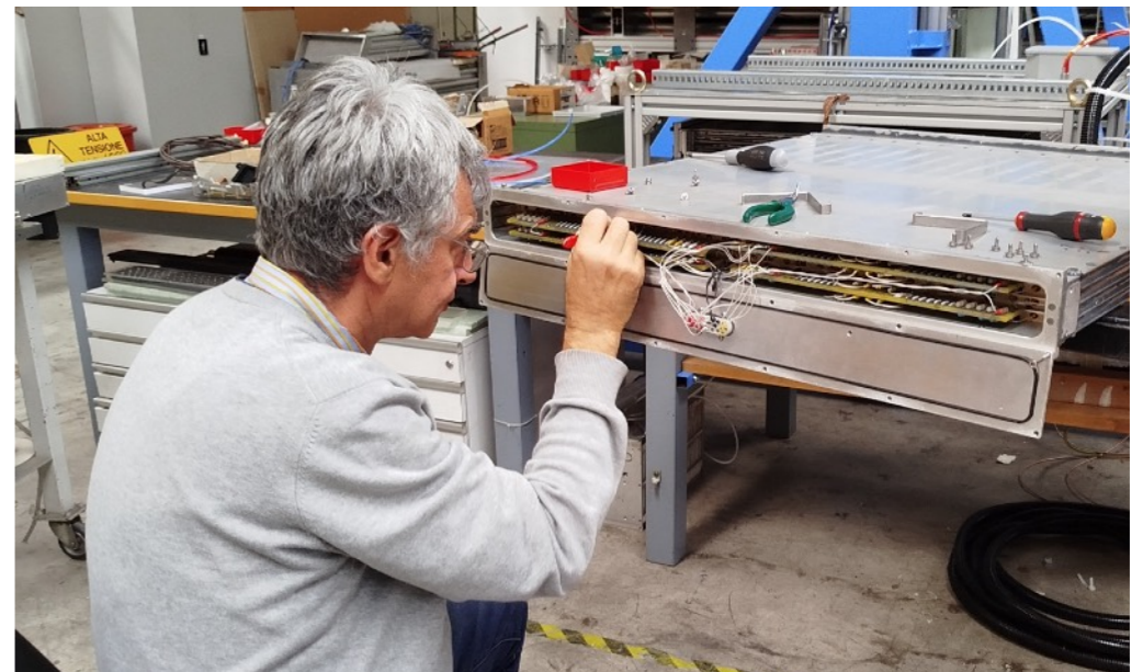
Franco fixing cathode pins
