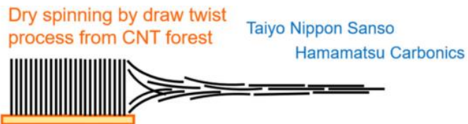
Figure 14. Dry spinning from a forest procedure schematics
