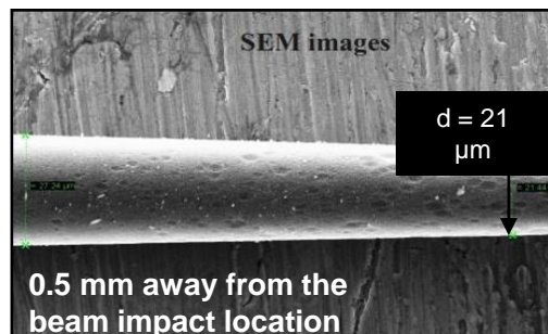
Figure 8. Aging Carbon Fiber (CF) after irradiation [3]
