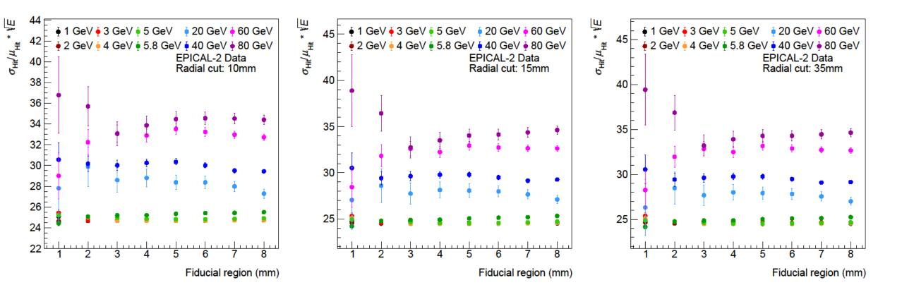
• The radial cut seems to have only a minor impact on the behavior of the resolution under fiducial region variation
