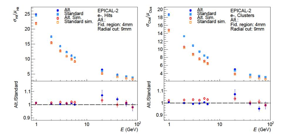
Resolution worsening not as bad as for the 8mm/5mm setting, except for 20GeV data (might be a statistical fluctuation)
