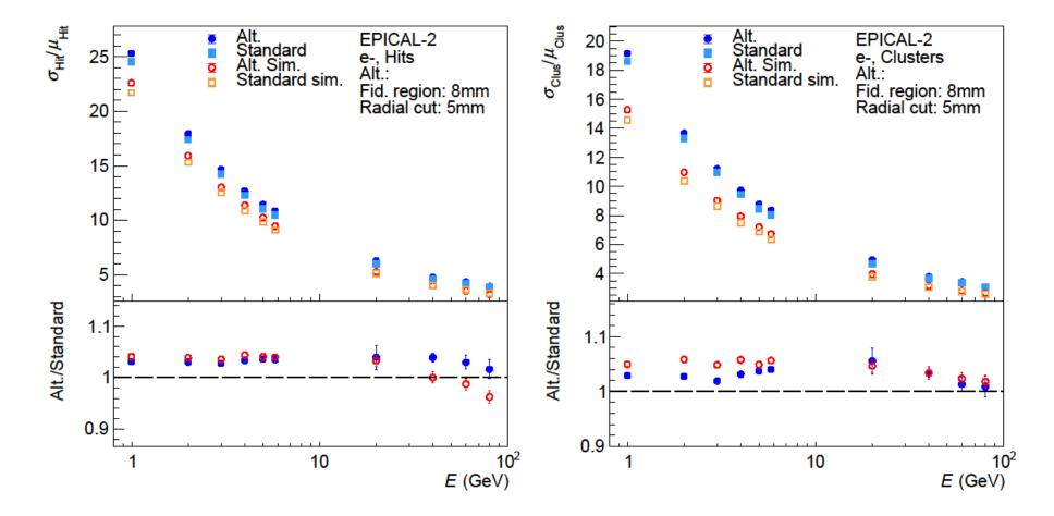
$\succ$  Resolution worsens by up to 5%, except for sim. at high energies
