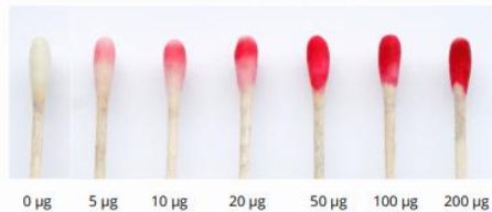
Figure 1. Results of the lead test with various amounts of lead.
