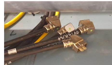
Figure 2 – Examples of recessed (unseated) pin
