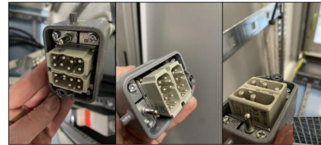
Figure 2 – Examples of recessed (unseated) pin
