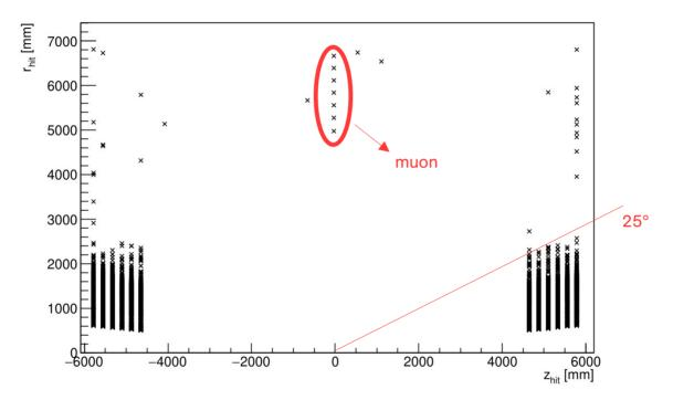
Muons can be identified by matching tracks to hits in the muon detectors.
