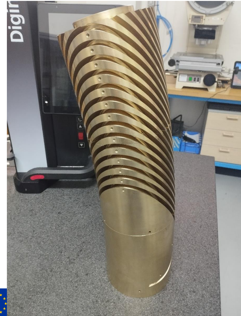
Assembly of #3 segments (inner former)
