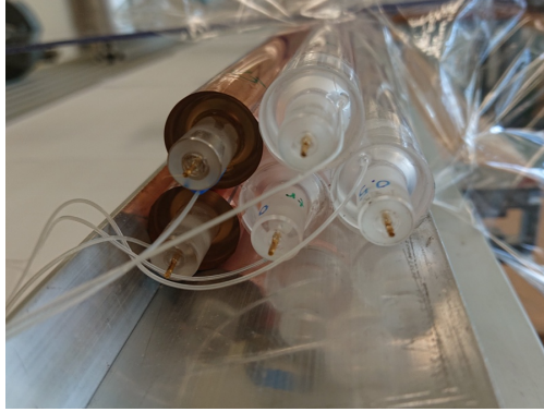
Figure 39: Prototype of the cemented pack design option with partly metalised tubes.
