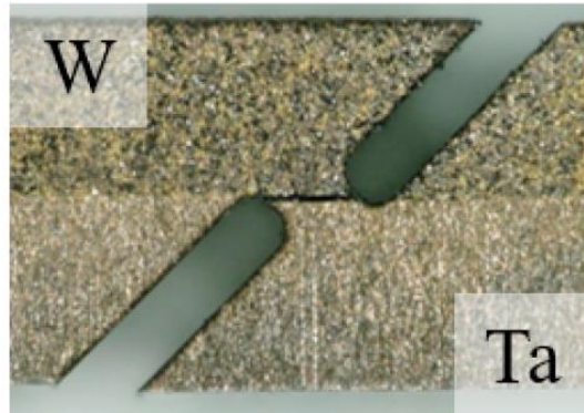
Fractured at interface before testing
