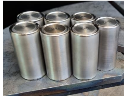
Capsules after EB welding
