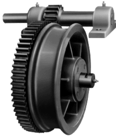
Figure 6 - Example of forbidden transmission system
