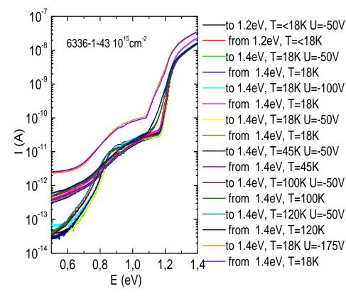
Both results confirmed the existence of the extended (macro) inhomogeneities in the irradiated Si (Its contribution depends on the bias)
