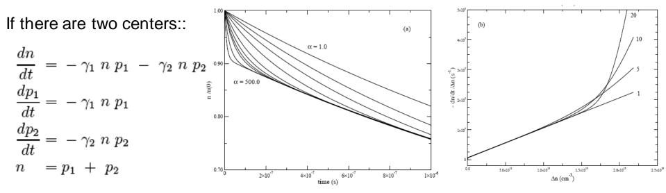
Additional centers introduce fast component in PC kinetics due to the nonlinearity
