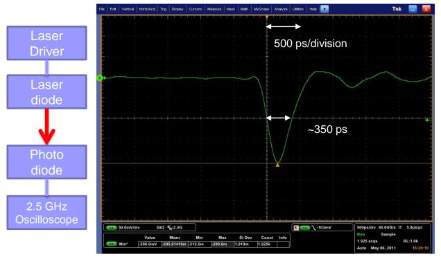
Parameters of the laser as measured with photodiode (real parameters are probably better)
