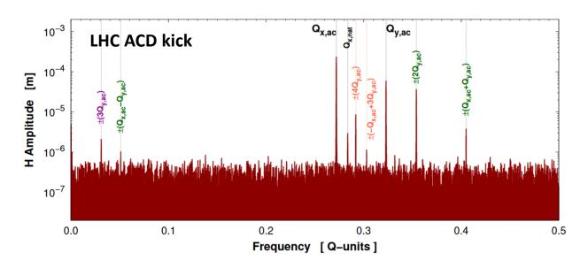
With RDT aim to quantify resonance strengths by how much they perturb turn-by-turn motion of excited beam
