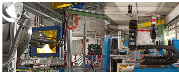
The HEARTS@GSI facility / Cave A showcasing a sample setup for electronics irradiation (left) and the current electronics target station (right). In the left picture the beam traverses from the left to right, exiting the vacuum exit window, through the beam monitors until it hits the devices under test. In the right picture the beam points towards the viewer. (Image: GSI)
