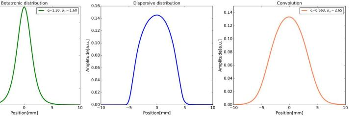
A **Gaussian fit** was then performed on both the generated betatronic distribution and the one obtained from the convolution, and the respective Gaussian sigma values were used to obtain the emittance.
