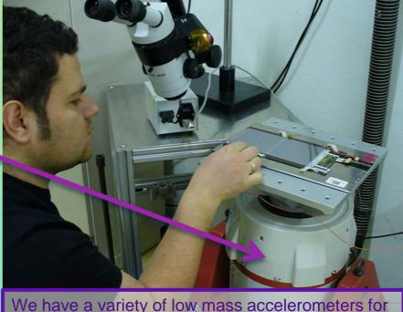
measurements on light-weight structures
