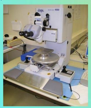
Shear testing is for checking die attach adhesion, bond wire adhesion and soldering quality for small components.
