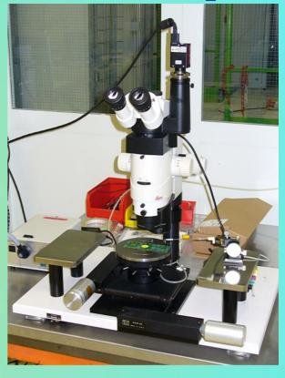
One high magnification stereo microscope with video camera. Three more stereo microscopes with lower magnification for routine inspection
