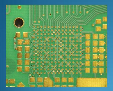
Mechanical attachement like screws shall be put away from BGA parts to avoid unnecessary load on solder joints
