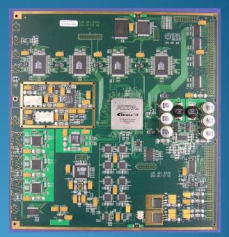
BGA parts should not be put in the middle of the board as it is where the max deflection will occur
