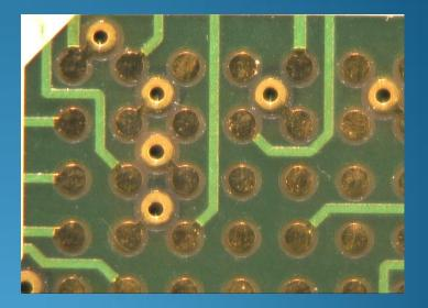
Vias close to BGA pads shall be tented to avoid solder wicking inside it and thus ensure homogene solder volume in joints
