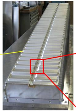
Thin (300 um) Alu shaped foil separates detector from primary LHC beam vacuum.
