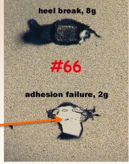
Improper metallization on PCB #1: Bond pads too narrow owing to over-etching, surface not flat, "bumpy", or like "Swiss cheese". Insufficient surface area of weld under bond foot leading to lifts during bonding or poor bond strength.
