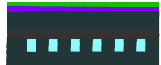
Monolithic CMOS detector with integrated micro-channels
