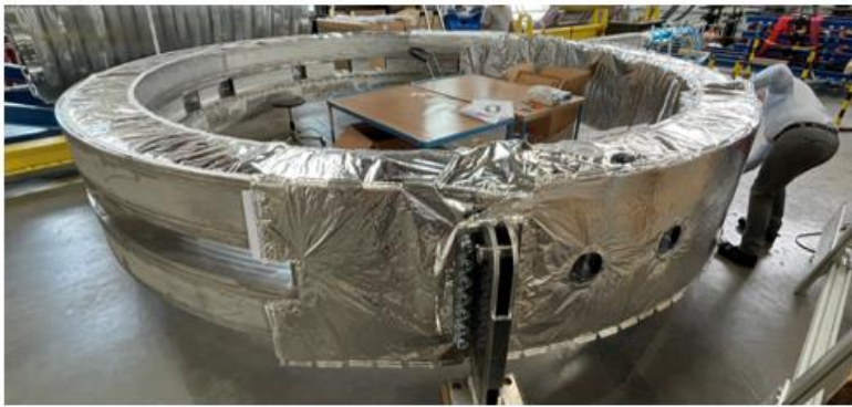
Outer vessel: equipped with radiation + N2 active cooldown
