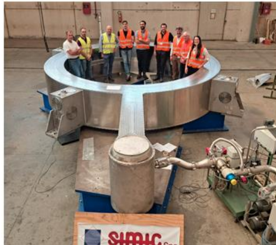
August 24: Cryostat vacuum (coils volumes) successfully tested at 10-6 mbar
