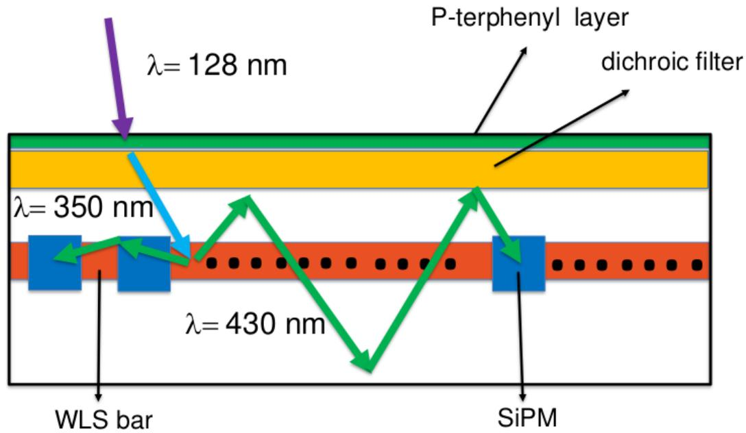
*Large area photon collector coupled to an array of SiPMs*
