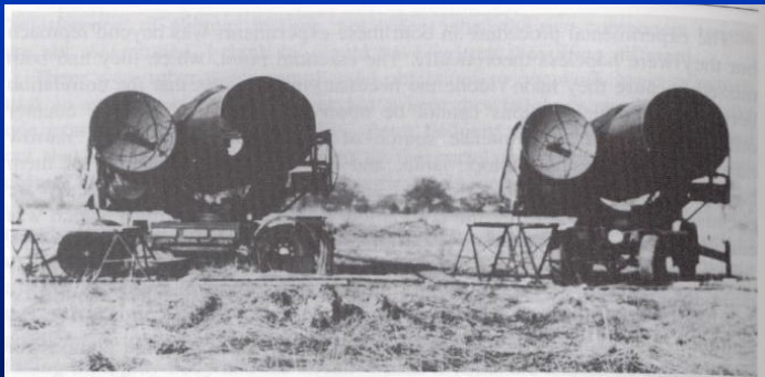
Figure 10.1 The first stellar intensity interferometer; the pilot model of the stellar intensity interferometer at Jodrell Bank in 1955. Two Army searchlights were used to make the first measurement of the angular diameter of a main sequence star (Sirius).
