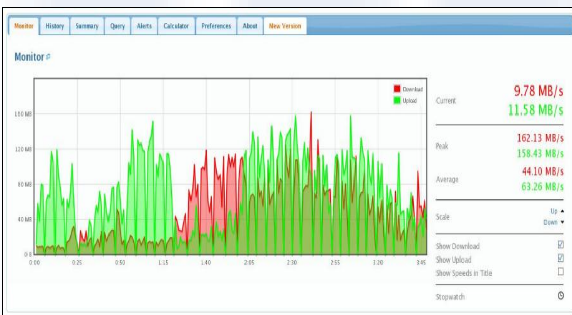
Network Usage when all the Nodes are involved 7 Jobs per Node Max rate 333MB/s
