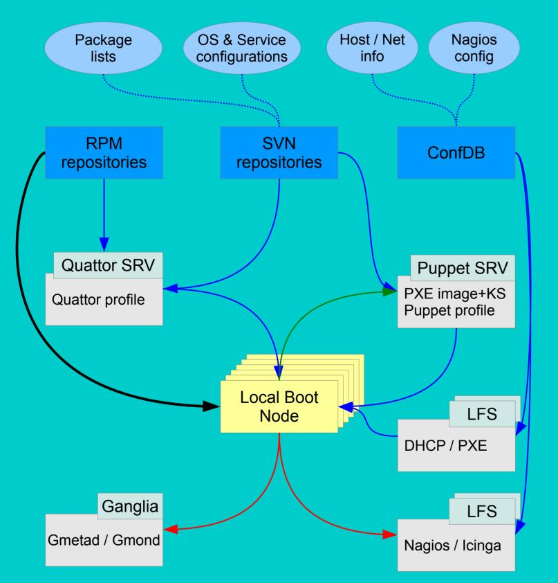
A node with locally installed OS receives configuration information from various sources (blue arrows); the Puppet server uses node status information (green arrow) to compile the profile. Its OS installation and updates are provided directly by the repository (black arrow). Monitoring information is collected by one of the Nagios servers and more detailed performance information is sent to the dedicated Ganglia server (red arrows).
