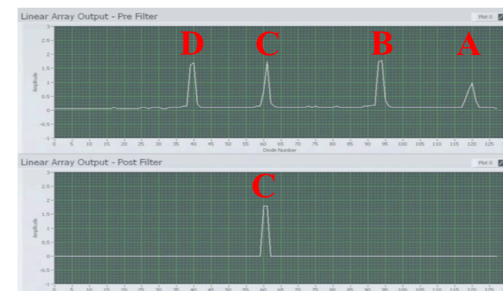
Fig 6c – Graphical representation photodiodes seeing IR light. The top graph is before the band-pass filter, the bottom is after.
