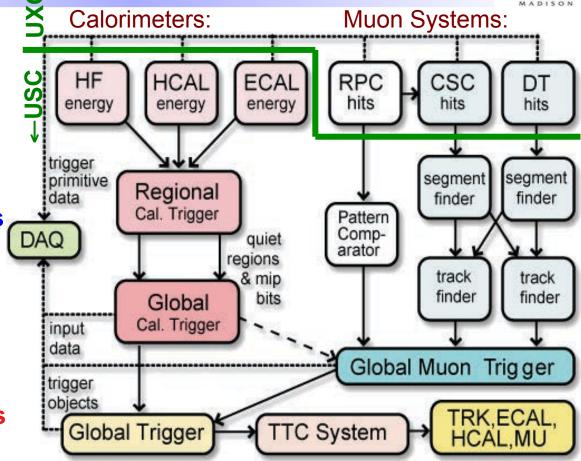
Generate L1A and send via TTC distribution to detector front-ends to initiate readout Maximum round-trip latency 4 µs
