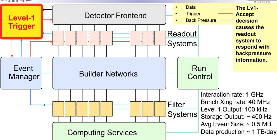
Lv1 decision is distributed to front-ends & readout via TTC system (red).
