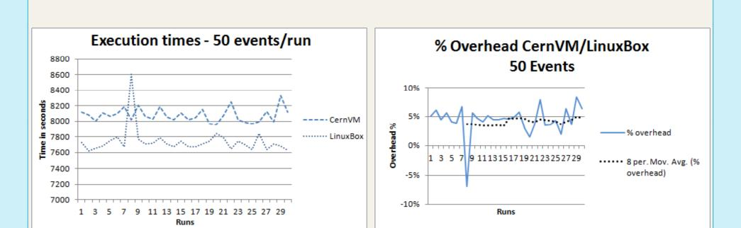
Based on the data represented by the above graphs, it is possible to see that the overhead due to the use of a Virtualizer is on the range of 4% to 6% when compared with a plain LinuxBox.
