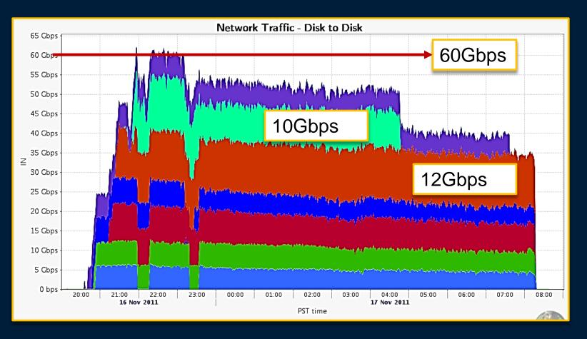
Disk write on 7 Supermicro and Dell servers with a mix of 40GE and 10GE Servers.
