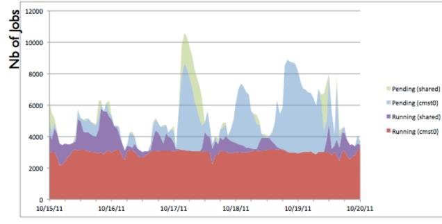
Even when all job slots were full, CPU utilization was only 70%. The memory footprint of the reconstruction executable was larger than expected and not all cores in each compute node could be used. CMS has since made improvements in memory consumption.
