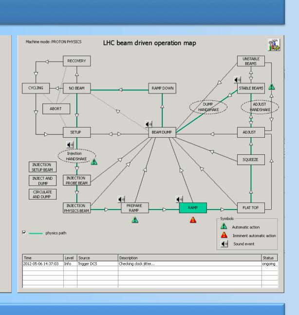
Automatization of routine operations will optimize ALICE efficiency by moving detectors READY, and guarantee the detector's safety by moving them SAFE, upon the relevant beam modes and conditions, and handshakes
