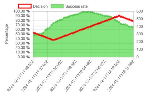
FTS failures during a short period of the test, overlaid with the 'decision' made by FTS on number of parallel transfers.
