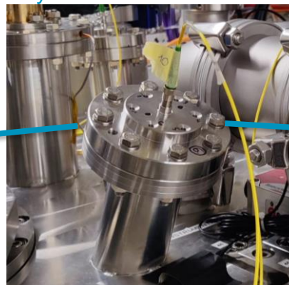
FSI Head (sensor) on the Cryomodule
