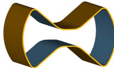
EBW seams: 40% pre-pass, 50kV 48mAmp 6 in/min beam speed Welding will be both sides to ensure the smooth surface inside
