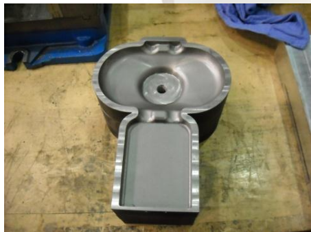
Finished first half with 4mm wall thickness
