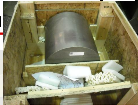
RRR>250 large grain Nb ingot
