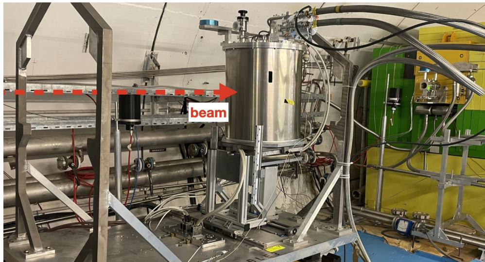
Vacuum vessel cooled to 4K impacted by beam in HRMT tunnel
