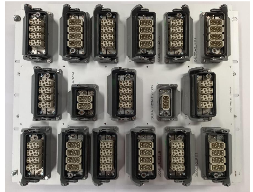
Back side: Input / Output current sensors / other racks
