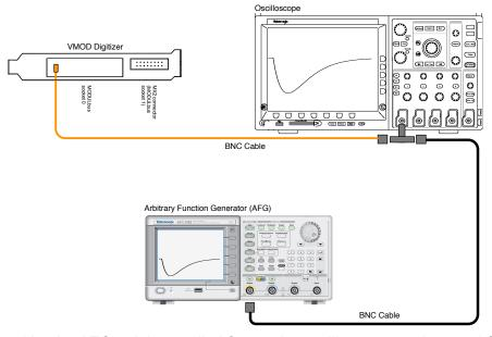
The signal generated by the AFG unit is supplied first to the oscilloscope, and passed from here to the Ch-0
