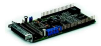
This has MODULbus form factor. It can be fitted into a PCI carrier card to be used in a regular PC. Its "vertical" resolution is 12 bit, and we know that the lower limit for the conversion time is 15 µsec. Let us assume that we sample every time a clock signal make a transition from negative to positive value as shown with "o" in the following figure.
