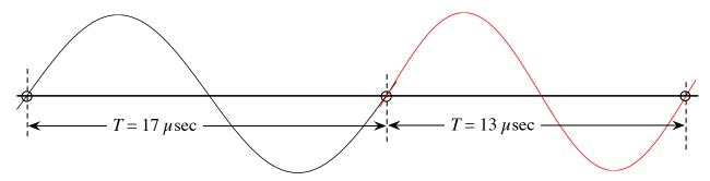
This may happen, and it is called "jitter". Also note that, this does not mean that "sampling frequency" is changing, because by "sampling frequency" we usually mean "the average sampling frequency."
