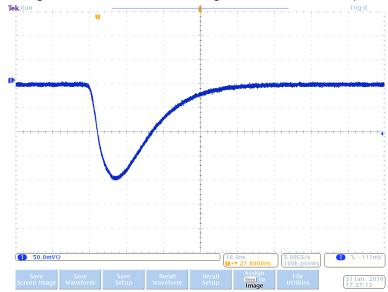
Arbitrary function generator is used to simulate a scintillator type pulse. It is extremely predictable and reproducible. We will use these pulses, and measure the time intervals from one pulse to the other.
