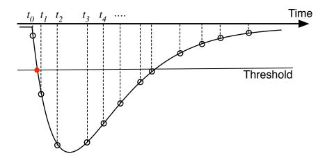
If we want to determine the time when the level of the signal is equal to a threshold value (from high to low), first, we have to find  $t_0$  and  $t_1$ , the time of two samplings in which that kind of transition happens, then, we interpolate the time of interest (red dot). At, this point the accuracy of sampling times become important.
