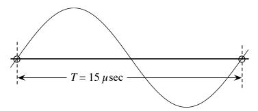
The question is how accurate is this timing? If this is accurate enough, our time resolution can be much better than the sampling period, once we interpolate our signal to find a specific time. Thus, our time resolution depends directly on the stability and reproducibility of this "clock". The sketch below is an example of changes in this "clock" signal from one period to another:
