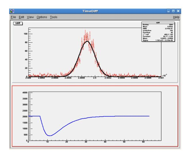
Perform a gaussian fit on the tdiff histogram, and note the fit parameters below:
