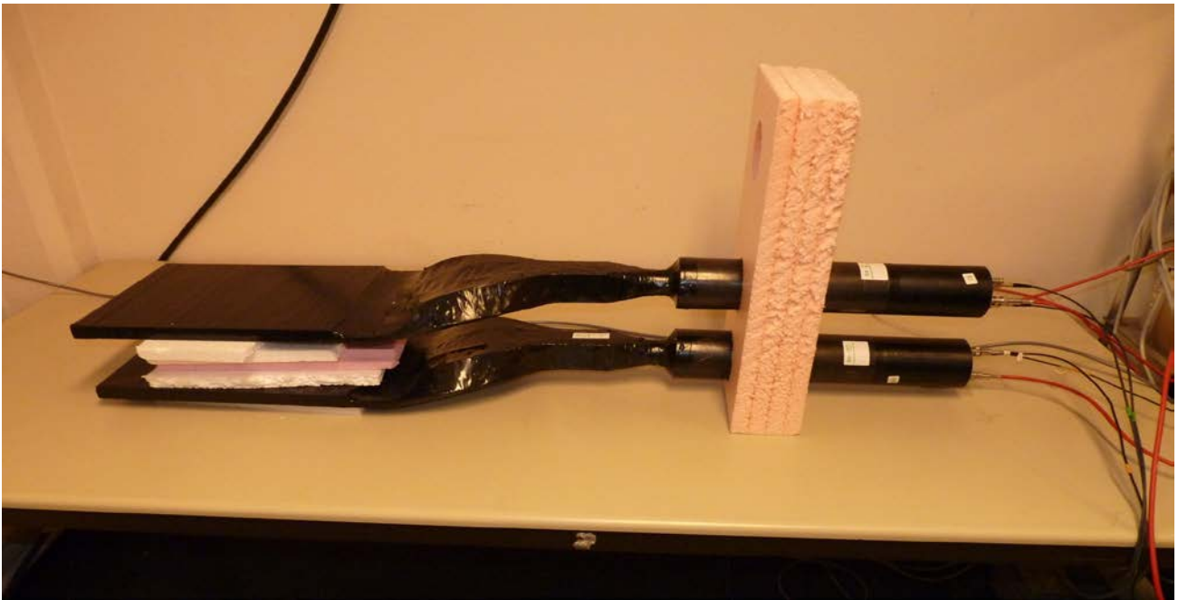
Figure 2. Scintillation counter setup
