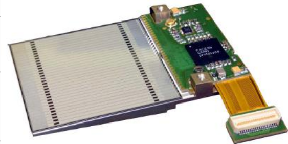
Fig. 5 The analog memory cell of PACE3
